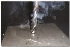
Stainless steel distorts up to 70% more than other steels when heat is applied, and therefore much more care should be taken when welding, cutting, and polishing.
